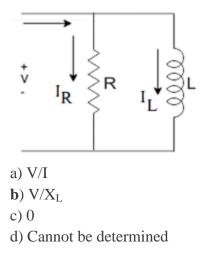
25. What is the phase relation between  $I_L$  and V from the following circuit?
