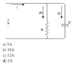
29. Find the value of IL if  $I_{C}{=}10\text{A}$  and  $I_{R}{=}6\text{A}.$
